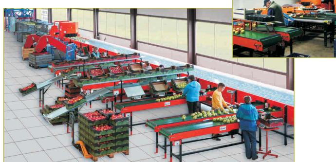
They are available in configurations with 2, 3, 4, 6 or 8 lanes resulting in capacities from ± 2.000 to 10.000 kg/hour. The positions of the size and spacer sections are detemined in accordance with customers' requirements.
