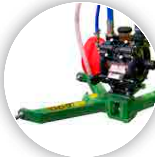
DRAWBAR The plant protection agent pump of all GSG trailermount machines is mounted on drawbar. This permits a maximum angle of turn without wide angle cardan shaft.
