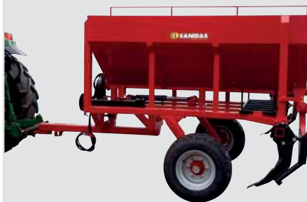
Λιπασματοδιανομέας SRT2 - L LARGE Fertilizer SRT2 - L LARGE
