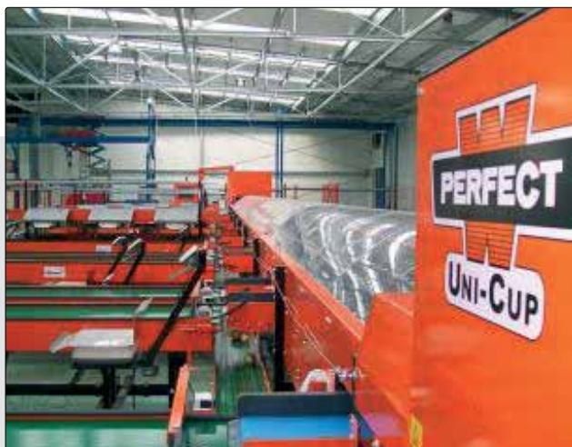
Διαλογητήριο PERFECT: UNI-CUP Sorting machine PERFECT: UNI-CUP
