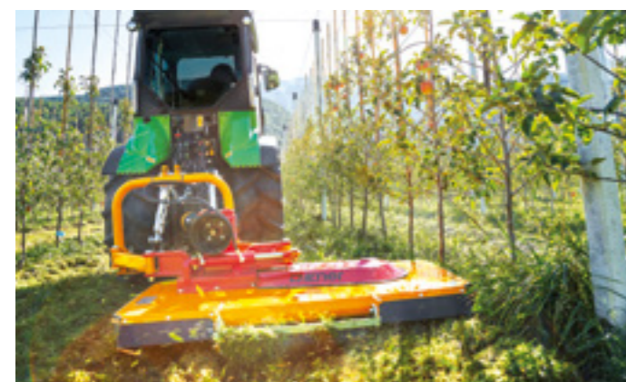
Wide offset! Allows centralized tractor passage throughout the orchard. Thanks to lateral grass discharge, the inter-row area is perfectly covered with the shredded mulch mass.
