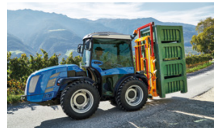
Valuable freight! The optional shock absorber protects the valuable harvest from impacts during transport.
